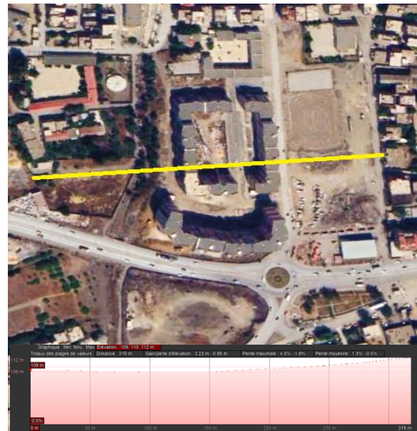
Figure III.25 : Section B-B sur in the field
