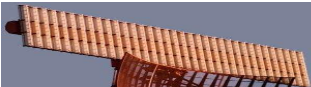
Figure II.4 Antenne du radar secondaire
