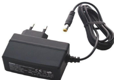
Figure 5.12.a 220v to 5v Alimentation
