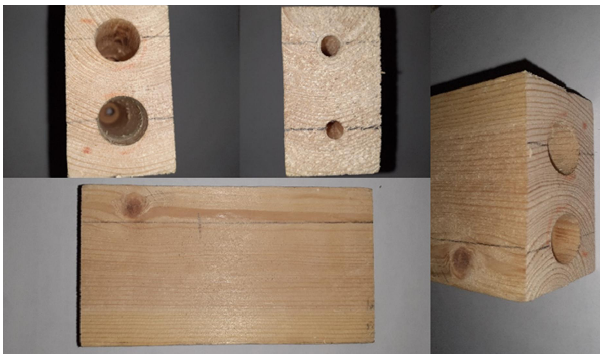
Figure 5.14 The Wooden Body of The Cannon
