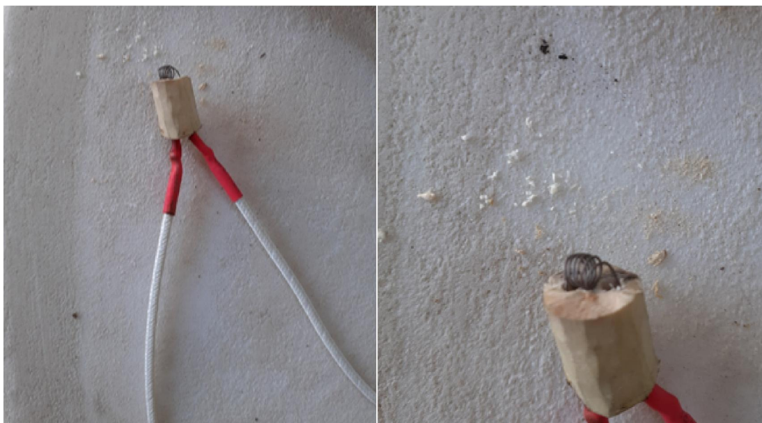
Figure 5.16 The Electric Firing System
