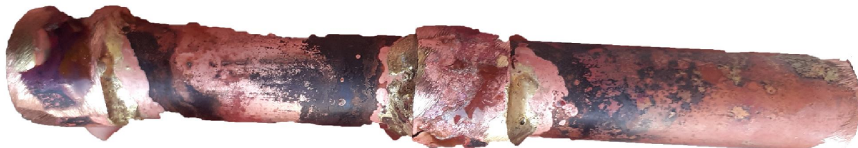
Figure 5.15 The Copper Tube with Rings Soldered into it
