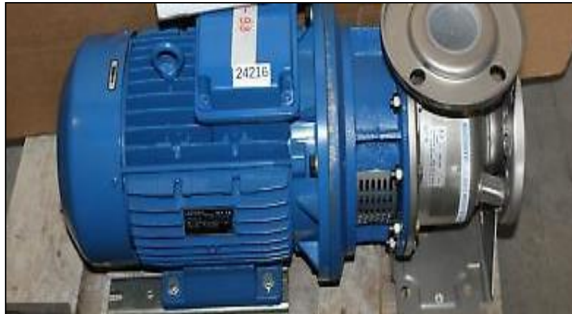
Figure III-4: Pompe jockey MOVITECH VF32-5 [29].
