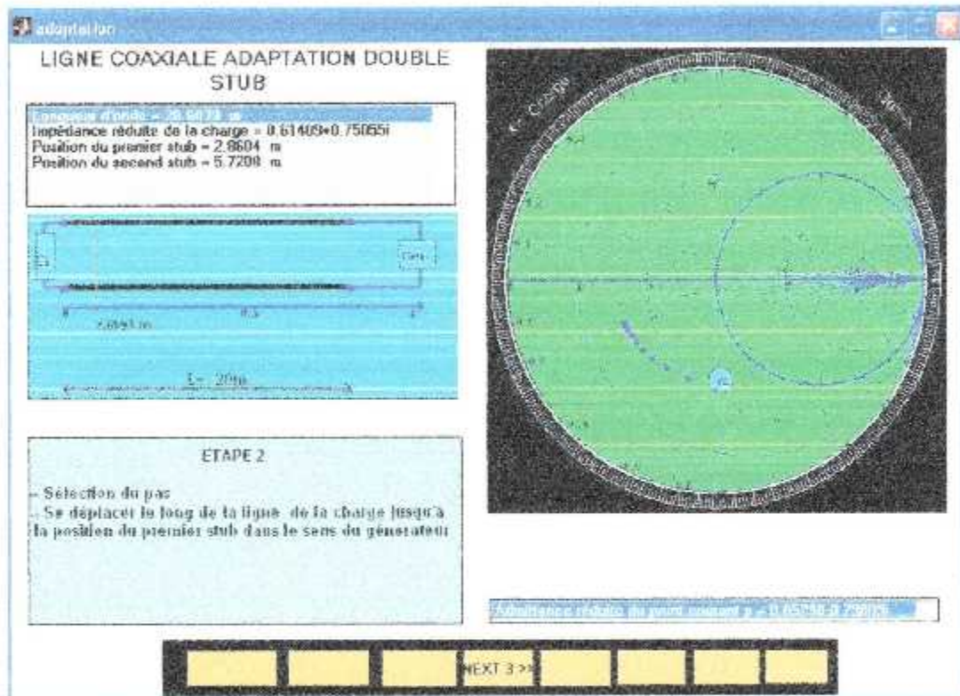
Figure V.17 : Adaptation deux stubs : Etape 2
