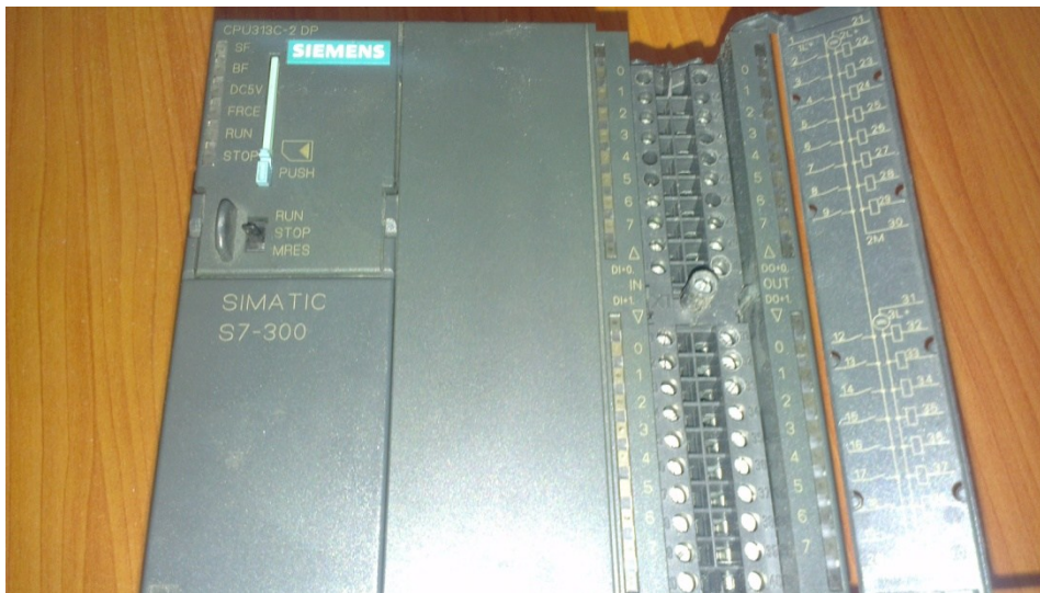
Figure 3.2 : Automate S7-300 2 C 2DP
