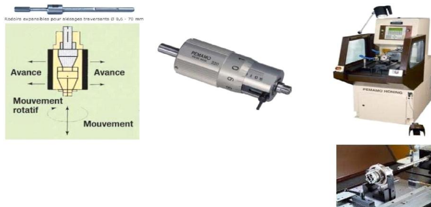
Figure 29: types de rodage [1]
