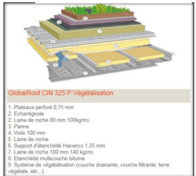
Figure 35 : les composants de GLOBALROOF CIN 325 P /source : http://ds.arcelormittal.com/construction/switzerland/systemes_solutions/globalroof/acoustique/cin_325_p/language/FR
