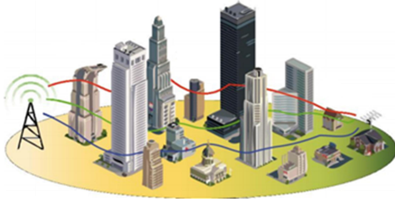
Figure 1.5: Multipath propagation in free space
