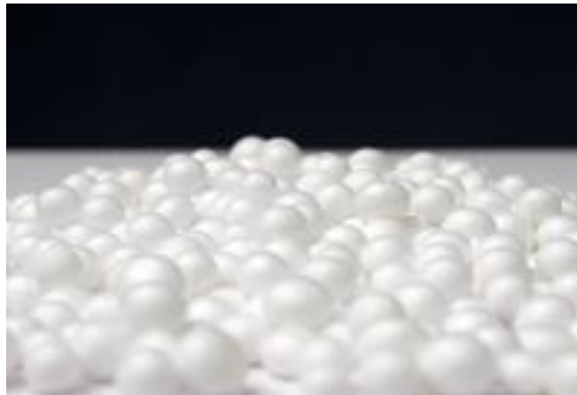
Figure I.2. Polystyrène expansé (EPS) [24]
