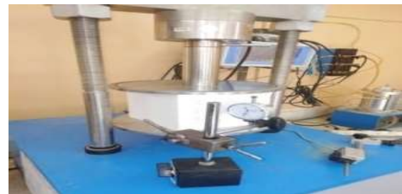
Fig.4 - Apparatus and direct compression test
