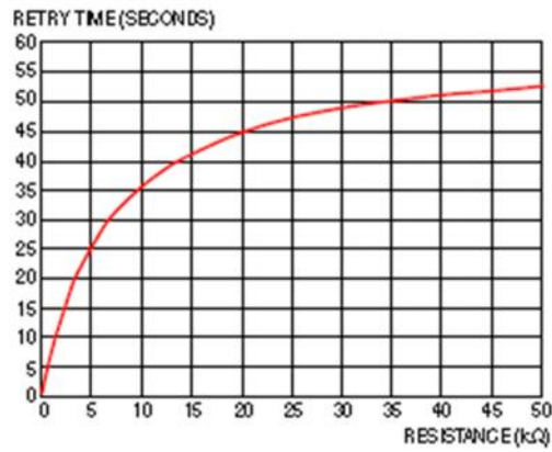
Figure 10. Fault Retry Time as a Function of the RRETRY Resistor
