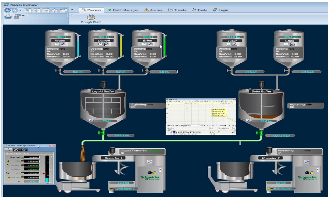
Figure 2.20 : Plateforme logiciel Vijeo Citect.
