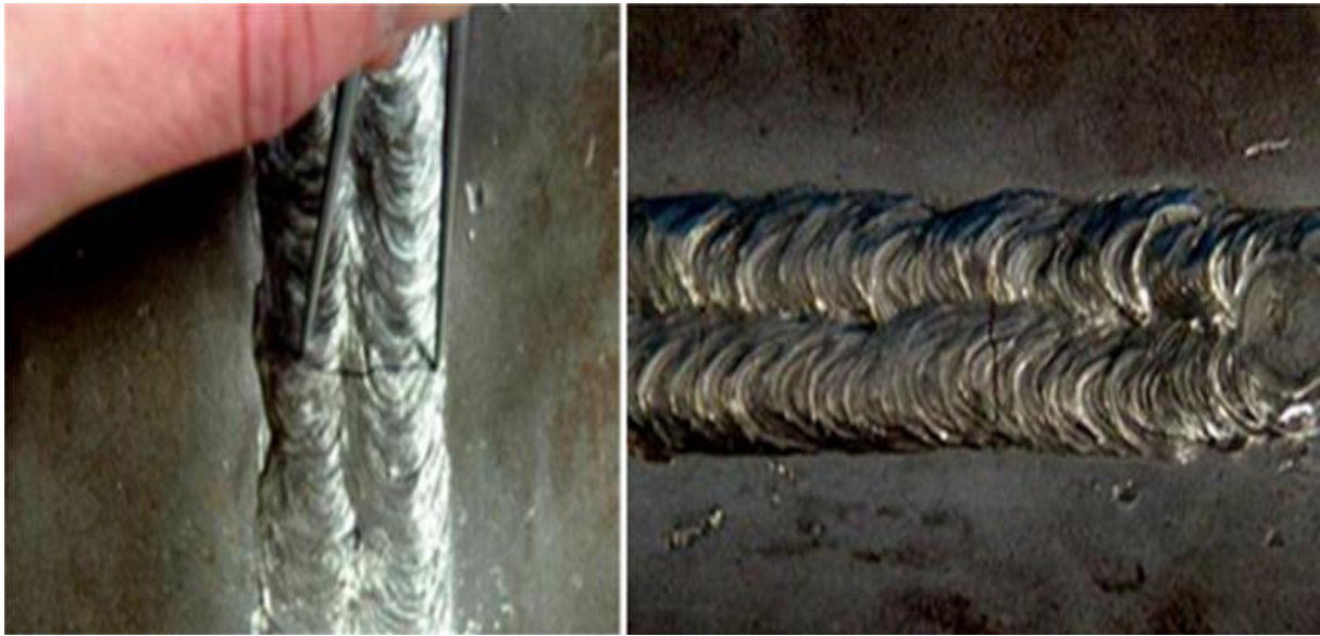
Figure 33: La fissure transversale.
