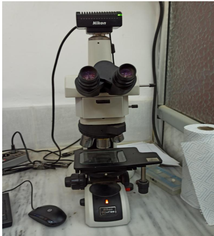
Figure III.12 : Microscope " Nikon Eclipse LV150N "
