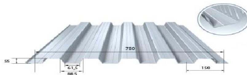
Figure I. 7: Bac d'acier type HI-BOND55-750.
