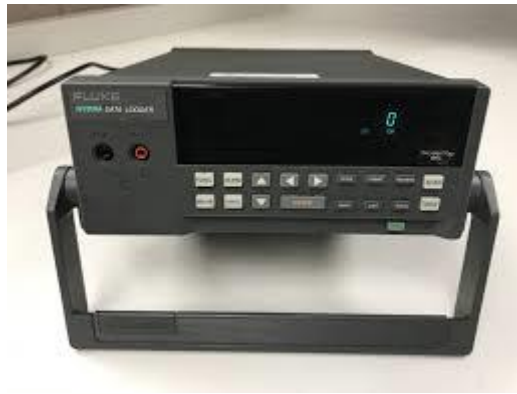
Figure 31: Data logger type Hydra 2700
