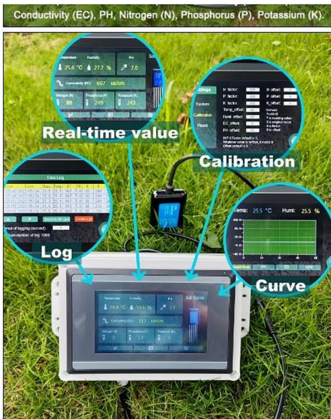
Figure 22 : Rapid Soil Sensor 7 in 1– ComWinTop. (Anonyme)
