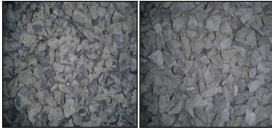
Natural coarse aggregate (Roughness and porosity: relatively low).
