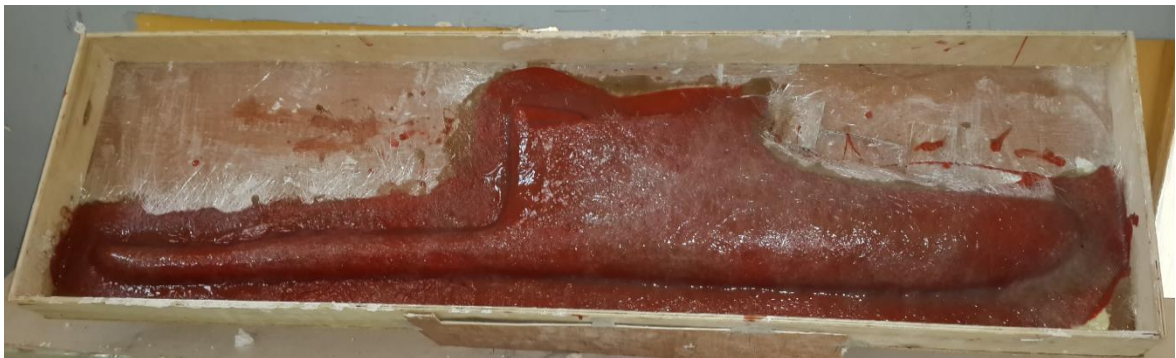
Figure (V-21) : Application de gelcoat.
