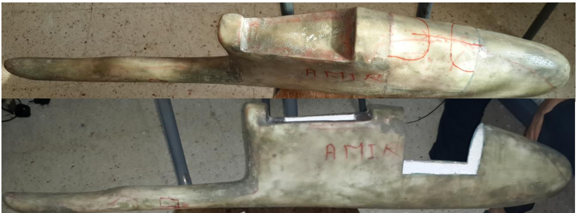
Figure (V-8) : Application de mastic de finition.
