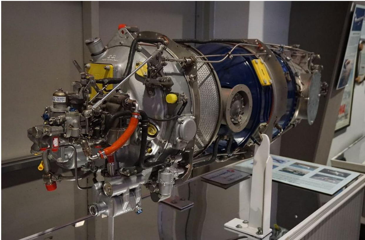
Figure 3.1: P&WC PT6 Turboprop Engine
