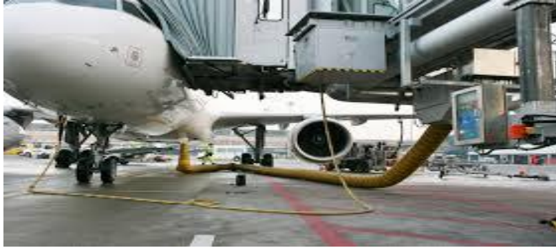
Figure4.5: Example of Preconditioned Air[9]
