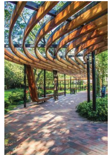
figure 134: Brise soleil en bois lamellé, source pinterest.com
