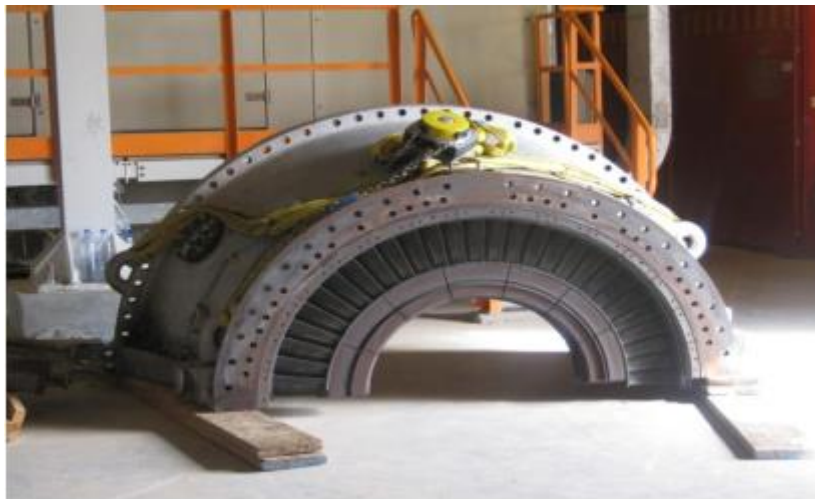
Figure I-3 : Ensemble stator de la turbine [2]
