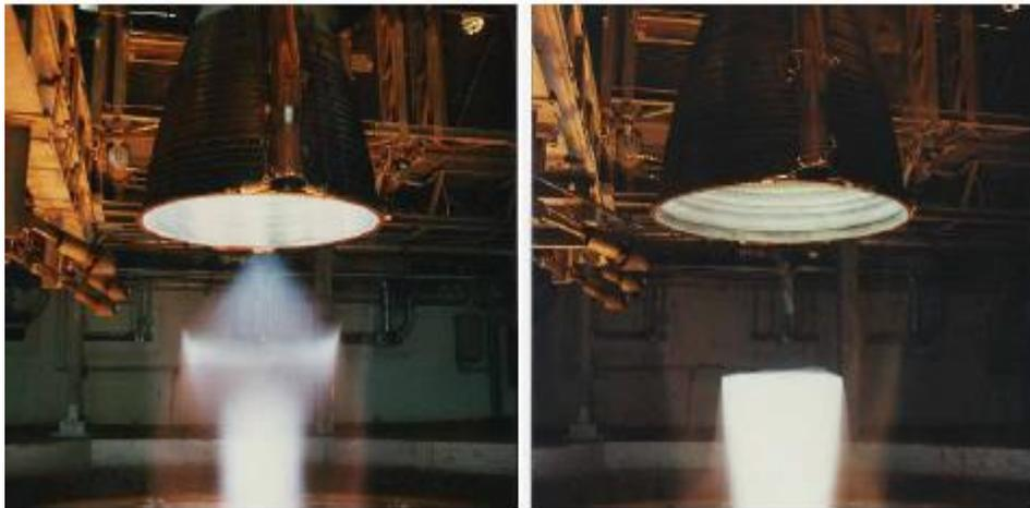
*Figure 1.18: Cap shock pattern (left) and Mach disk (right) in the plume of the Vulcain engine [4]*
