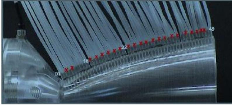
*Figure 3.1: Acrylic glass TIC nozzle with transducer ports [1]*
