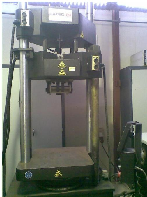
**Figure IV.9:** Machine de traction
