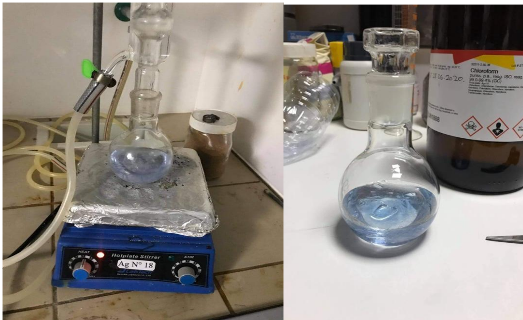
Figure 2.15 : Extraction solide/liquide du PET.
