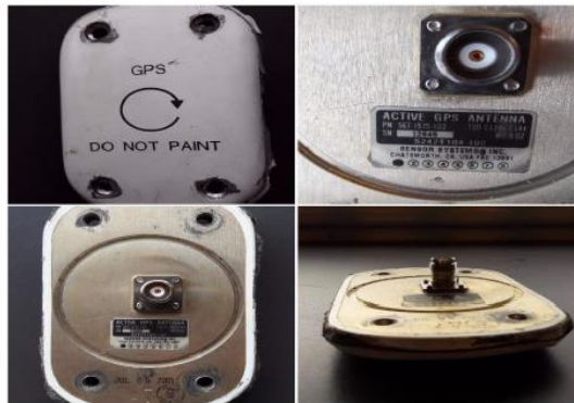
Figure I.27: Active GPS antenna S67-1575-133
