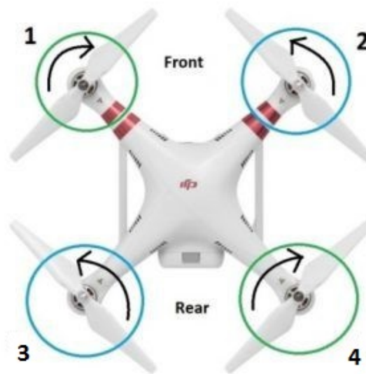
Figure II.2: Direction of propeller's rotations [40].
