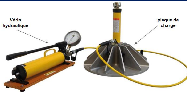
Figure I.5.6 photo vérin hydraulique et plaque de charge
