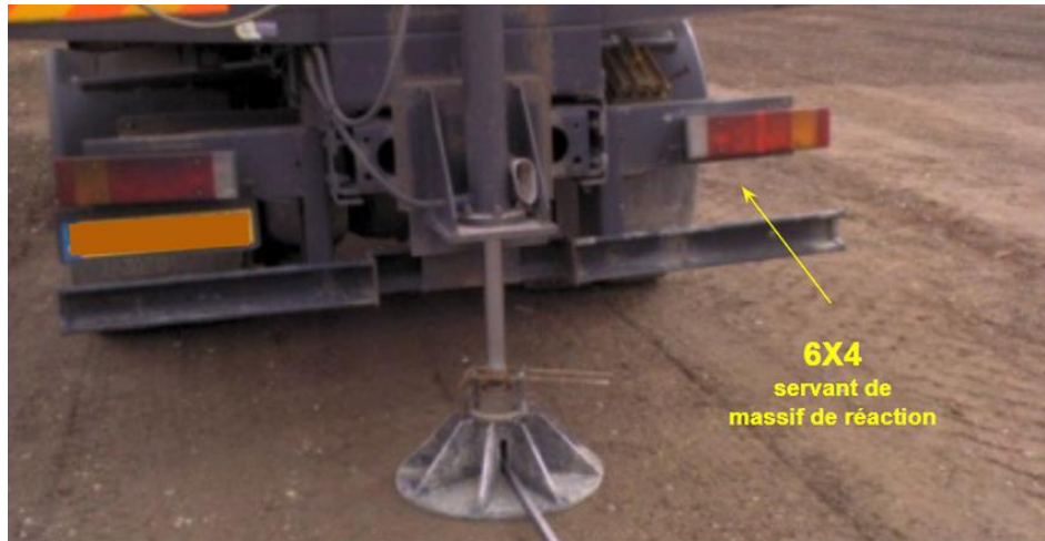
Figure I.5.4 photo essai à la plaque
