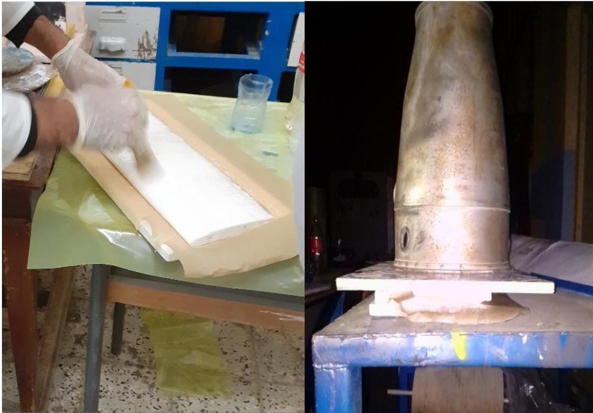
Fig (IV-26) Attaching Glass Fibers to the Wing Surface.
