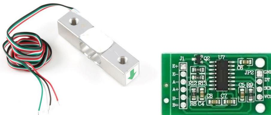
Fig (IV-3). Load cell (left), and electronic module of load cell (right).
