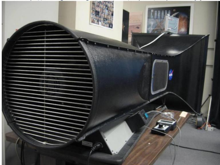
Fig (I-5). The Diffuser of a Pitsco AirTech Tunnel (NASA)
