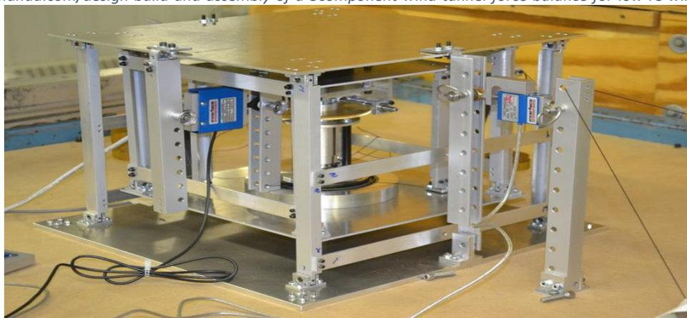
Fig (I-13). Full-Scale Wind Tunnel Force Balance for Lift and Drag measurement.
