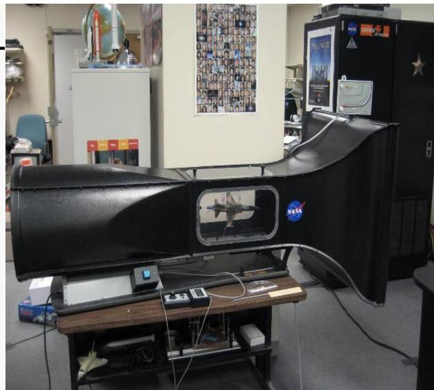
Fig (I-1). Low-Speed Closed Tunnel (NASA)
