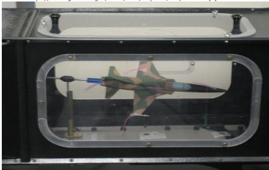
Fig (I-4). model of an F-5 fighter in the Test Chamber of a Pitsco AirTech Tunnel (NASA).
