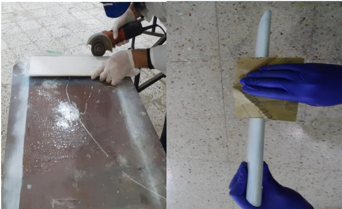
Fig (IV-27) Impurities Removal and Polishing Process.
