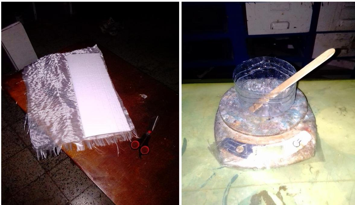
Fig (IV-25) Preparation of the Glass Fiber and Epoxy Mixture and the Matrix.
