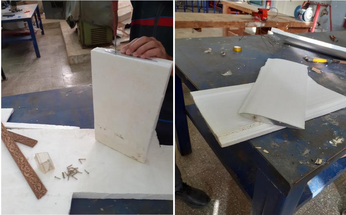
Fig (IV-24) The Process of Shaping the Wing.
