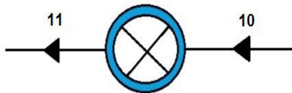
Figure (III.9): Pompe d'extraction
