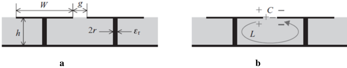
Figure 13: LC model for the mushroom-like EBG structure ; (a) EBG parameter ,(b) model LC.
