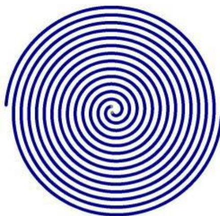
Figure 8: Representation of spiral antenna (11).
