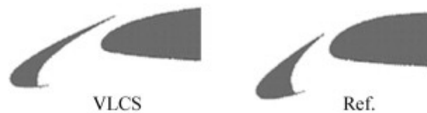
Figure 2-10 VLCS: very long chord slat
