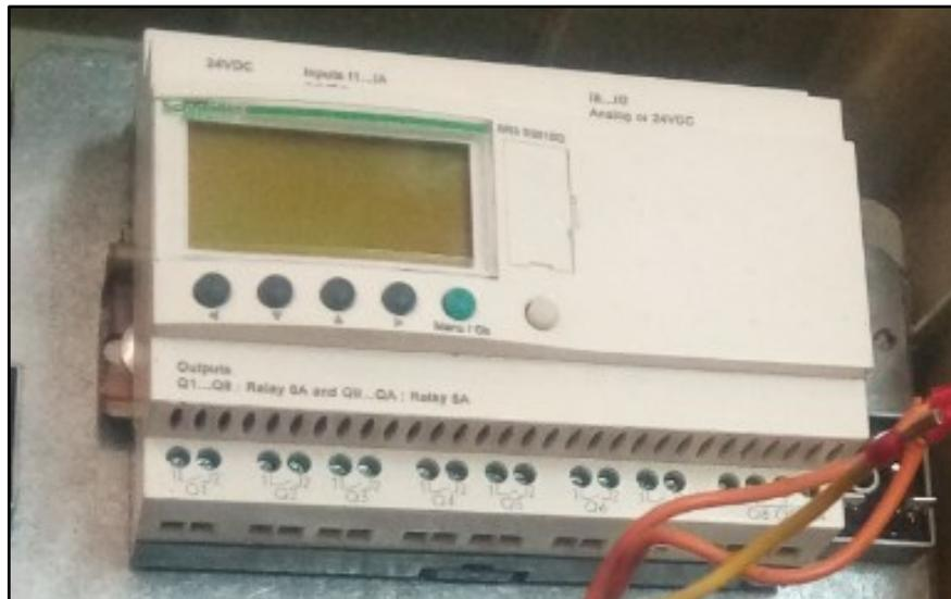
**Figure II.11:** Automate programmable Zelio de type SR3 B261BD
