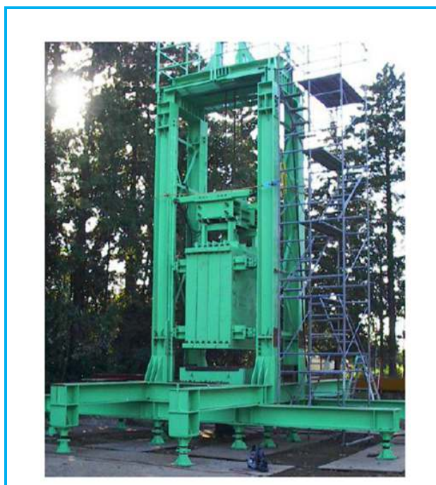
Figure I-18 : Essai Hybridynamic 70 tonnes [6]
