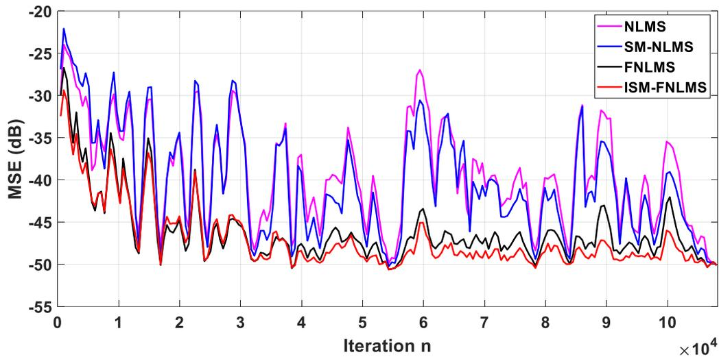
**Figure.2.21.** MSE evaluation Input: Speech signal with VCN system of length  $L = 1024$ . Output noise: SNR=50dB.
