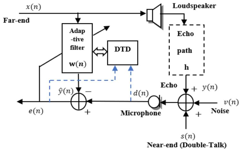
Figure.3.2. Basic structure of the AEC with DTD based on NCC.
