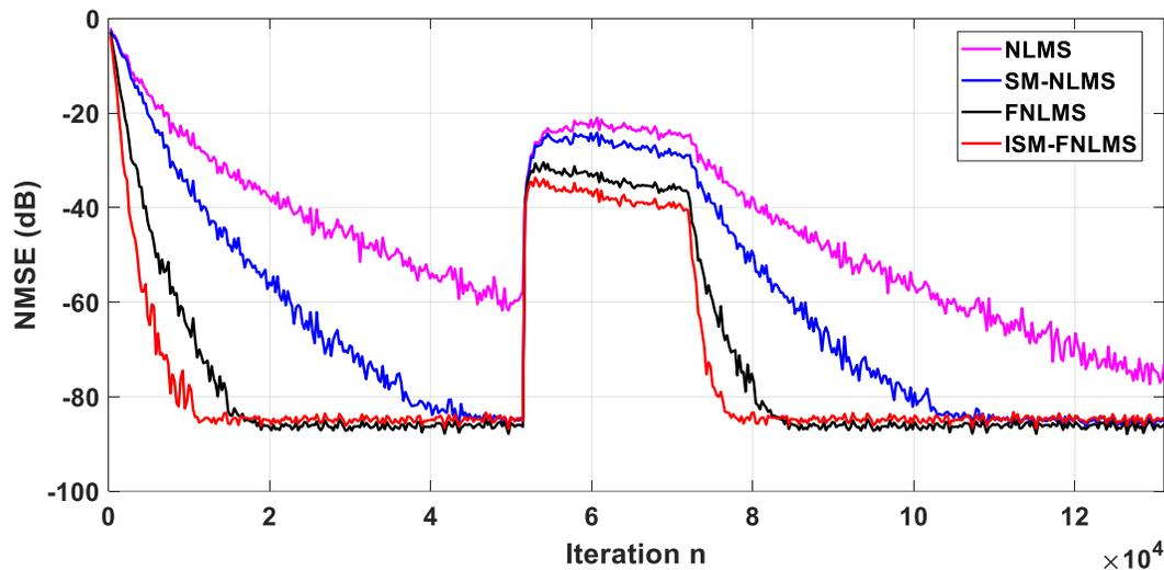
**Figure.2.18.** Comparison of tracking time-varying system of length  $L = 256$ . Input: USASI noise. No output noise.
