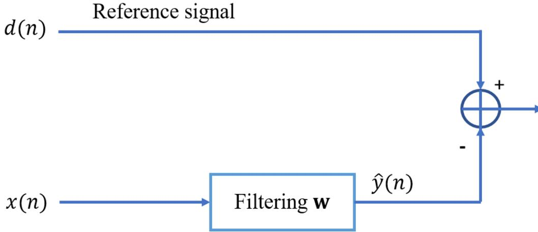
**Figure 1. 8:** Wiener filtering scheme.
