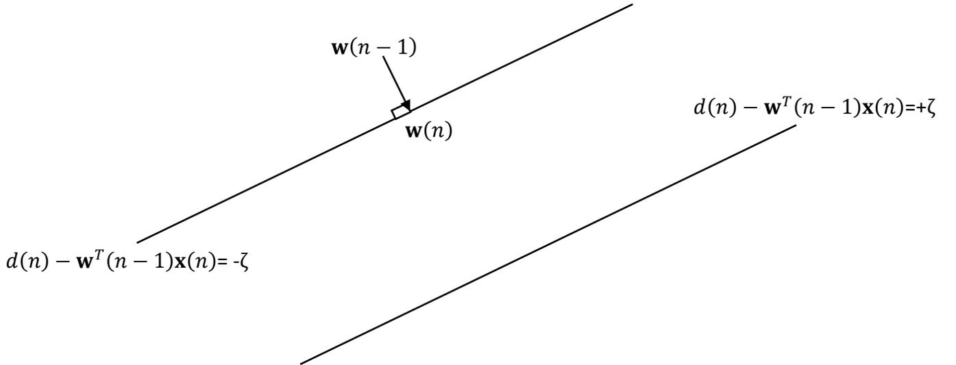
**Figure 2.1:** Coefficient vector updating for the SM-NLMS algorithm.
