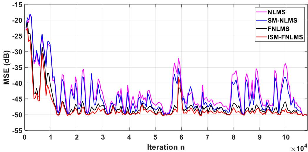
**Figure.2.20.** MSE evaluation Input: Speech signal with car system of length  $L = 256$ . Output noise: SNR=50dB.
