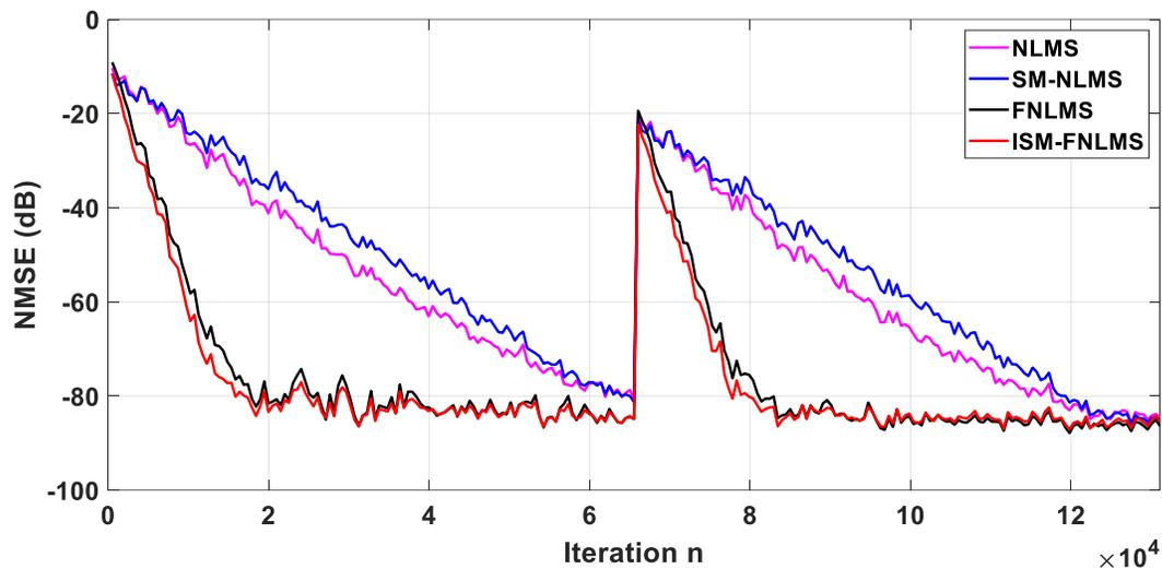
**Figure.2.16.** Comparison of the initial convergence and the re-convergence after an abrupt change in the impulse response of VCN system of length  $L = 1024$ . Input: USASI noise. No output noise.
