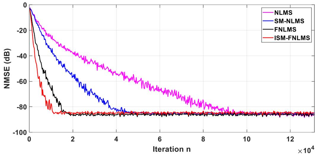
**Figure.2.11.** Comparison of the initial convergence and the SS-NMSE. Input: USASI signal with Car system of length  $L = 256$ . No output noise.
