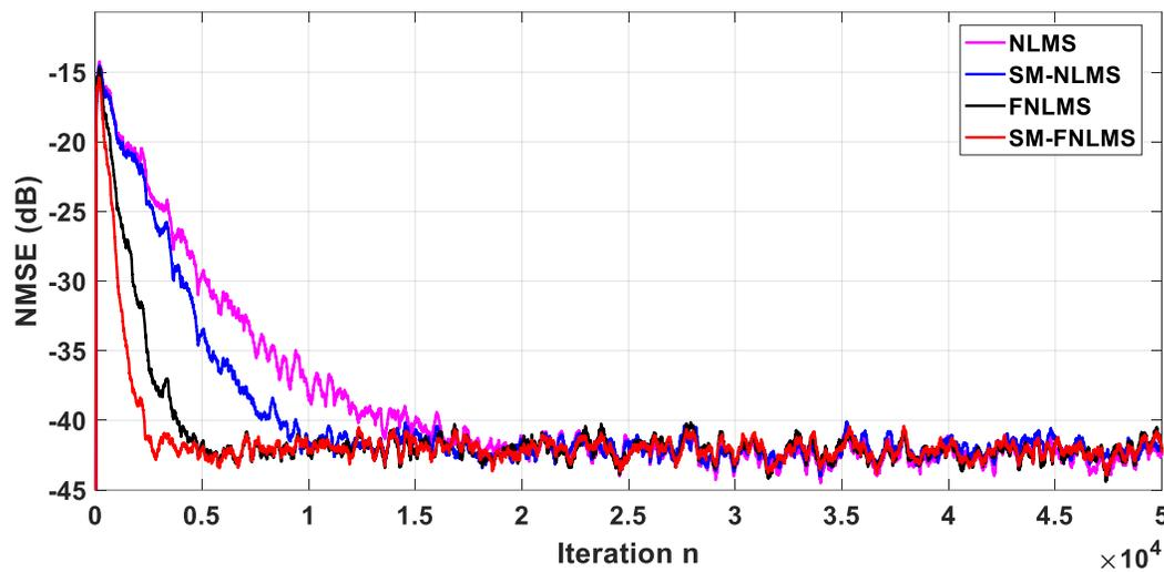
**Figure.2.5.** The Comparison of the initial convergence and the steady-state NMSE. Input: USASI signal with Car system of length  $L = 1024$ . SNR=50 dB.
