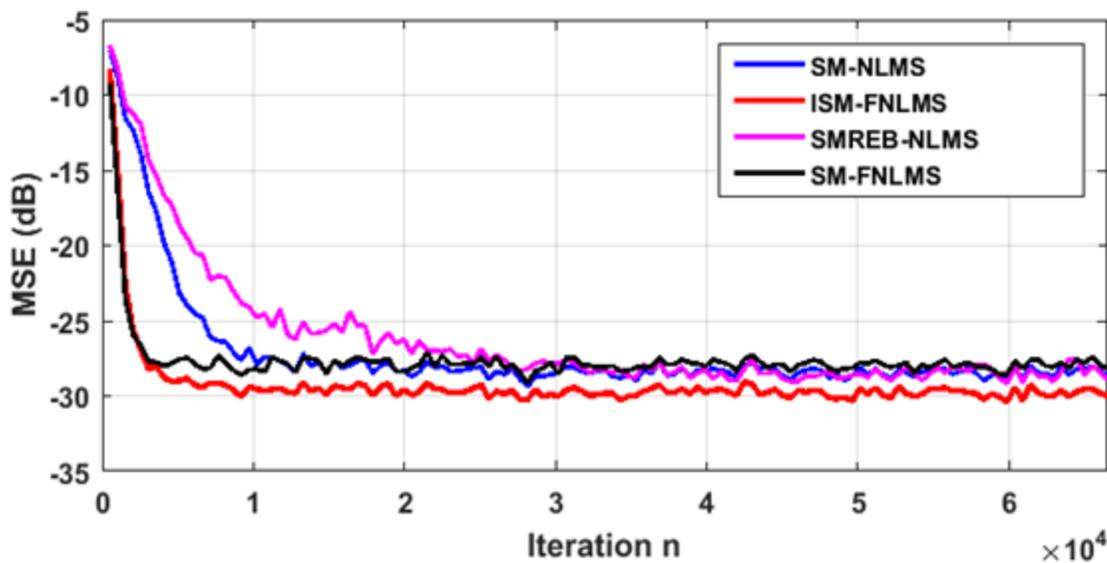
**Figure.2.22.** Comparison of SM algorithms with car system of length  $L = 256$ . Input USASI noise. Output noise: SNR=30dB. Threshold  $\zeta = 0.025$ .
