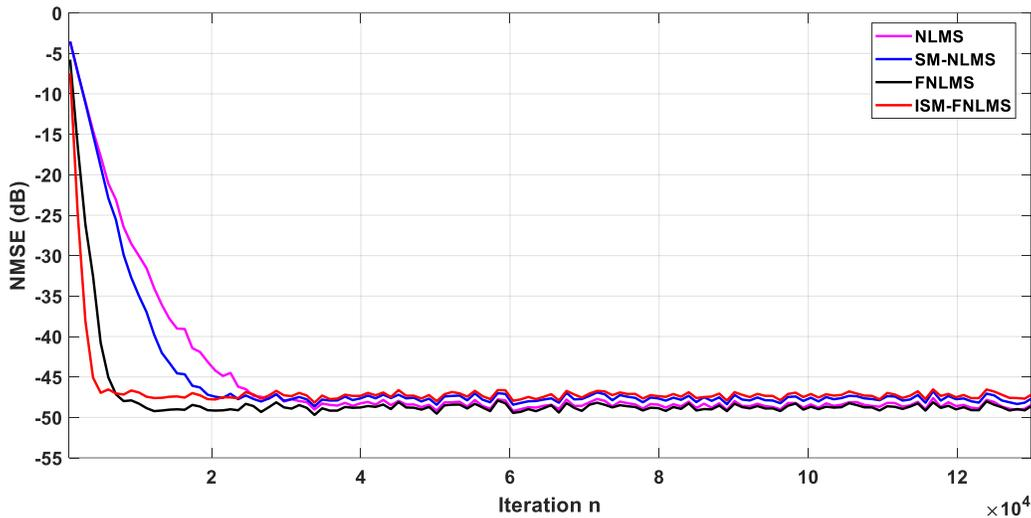
**Figure.2.14.** Comparison with noisy input: USASI signal with car system of length  $L = 256$ . Output noise: SNR=50 dB. Threshold  $\zeta = 0.0032$ .  $\sigma_y^2 = 0.38$ .
