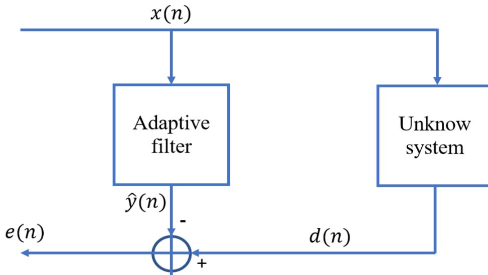
**Figure 1. 4:** The bloc diagram of system identification.
