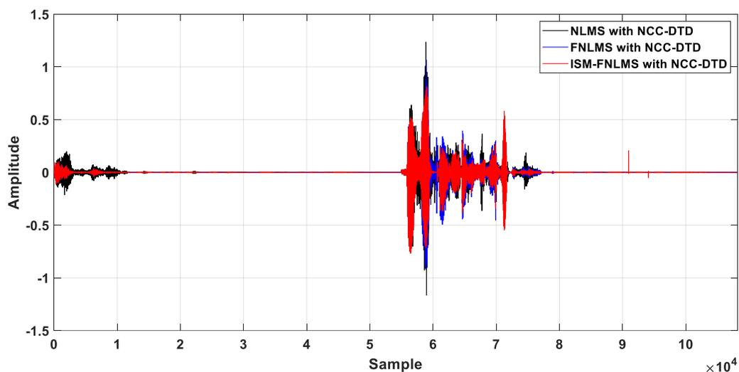
**Figure.3.7.** Output waveforms of ISM-FNLMS, FNLMS and NLMS with DTD in car system of  $L = 256$ .
