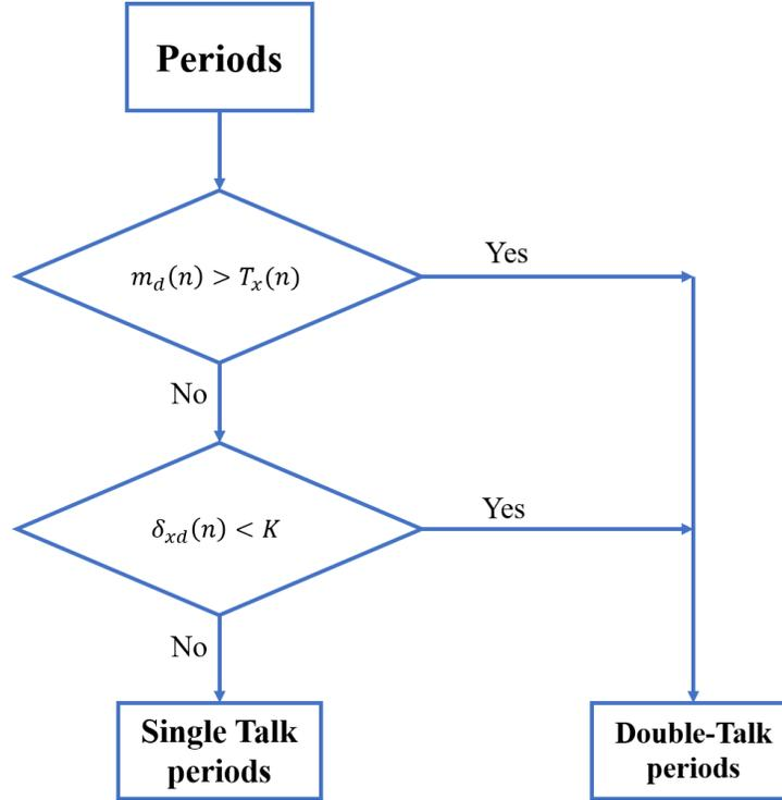
**Figure.3.4.** The flowchart of the DTD based on joint signal energy and cross-correlation estimation [59].
