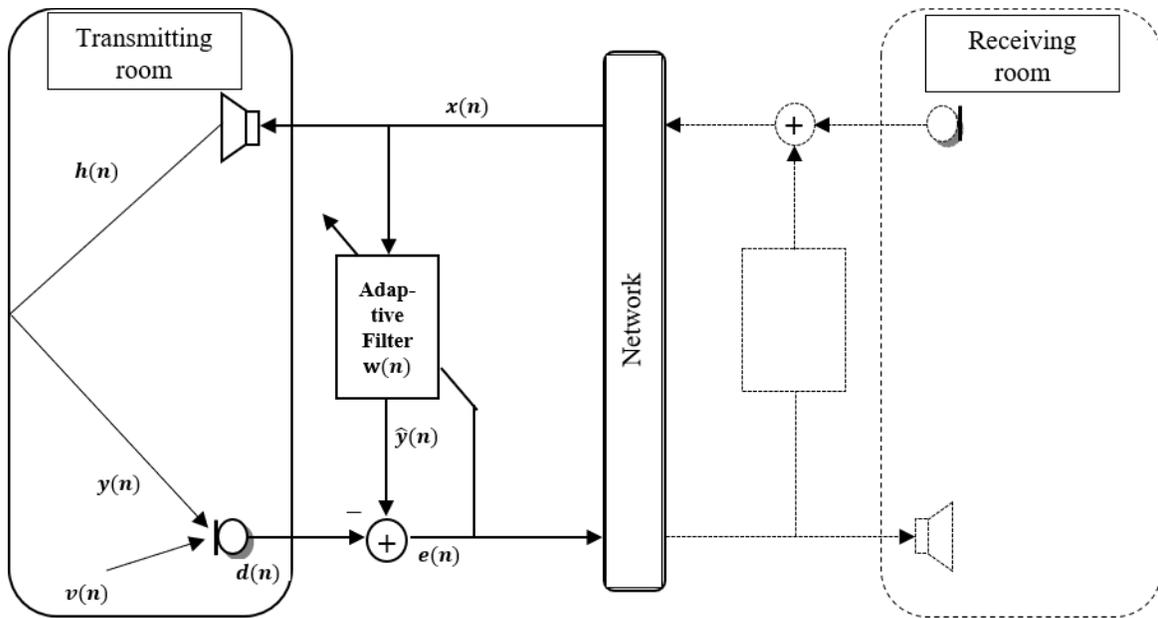
**Figure.1.2.** Basic AEC setup in a teleconferencing system.
