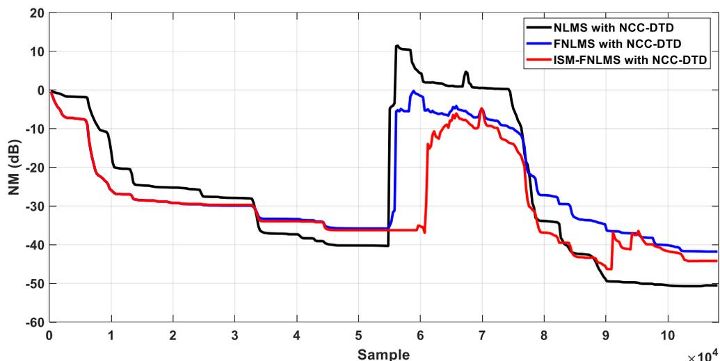
**Figure.3.6.** NM of ISM-FNLMS, FNLMS and NLMS with DTD in car system of  $L = 256$ .
