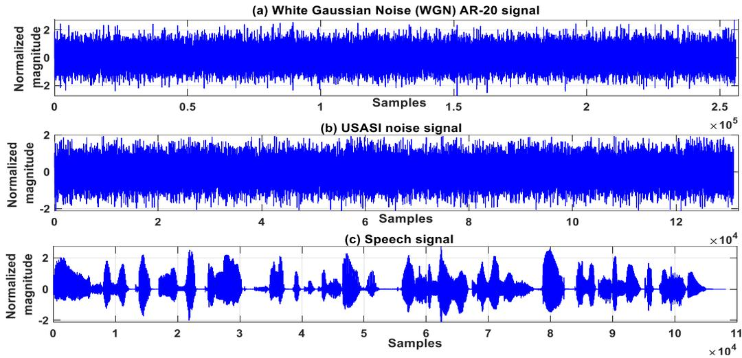
**Figure.2.2.** The used normalized input signals. (a) WGN AR-20 signal with a length of 256000 samples, (b) USASI noise signal with a length of 131072 samples, (c) Speech signal with a length of 108208 samples.
