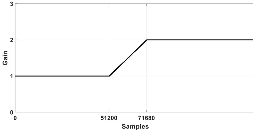
**Figure.2.17.** Variable artificial gain used for the tracking experiment. The variation is made between  $n = 51200$  and  $n = 71680$ .
