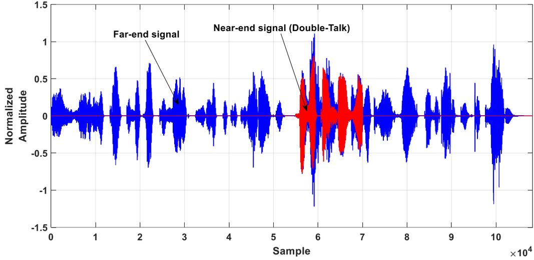
**Figure.3.5.** The used signals,  $x(n)$ : Far-end signal (in Blue),  $s(n)$ :Near-end signal DT (in red).
