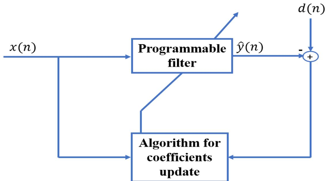
Figure 1. 3 : Principle of an adaptive filter.
