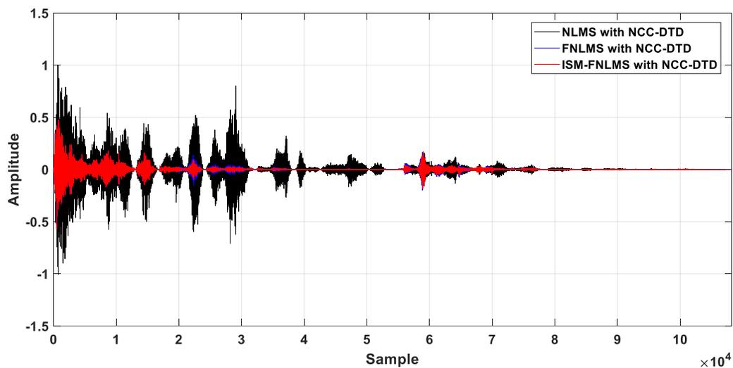
Figure.3.9. Output waveforms of ISM-FNLMS, FNLMS and NLMS with DTD in VCN system of  $L = 1024$ .
