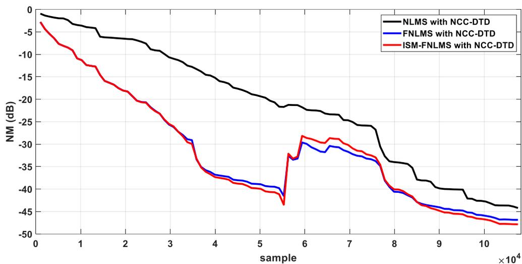
Figure.3.8. NM of ISM-FNLMS, FNLMS and NLMS with DTD in VCN system of  $L = 1024$ .
