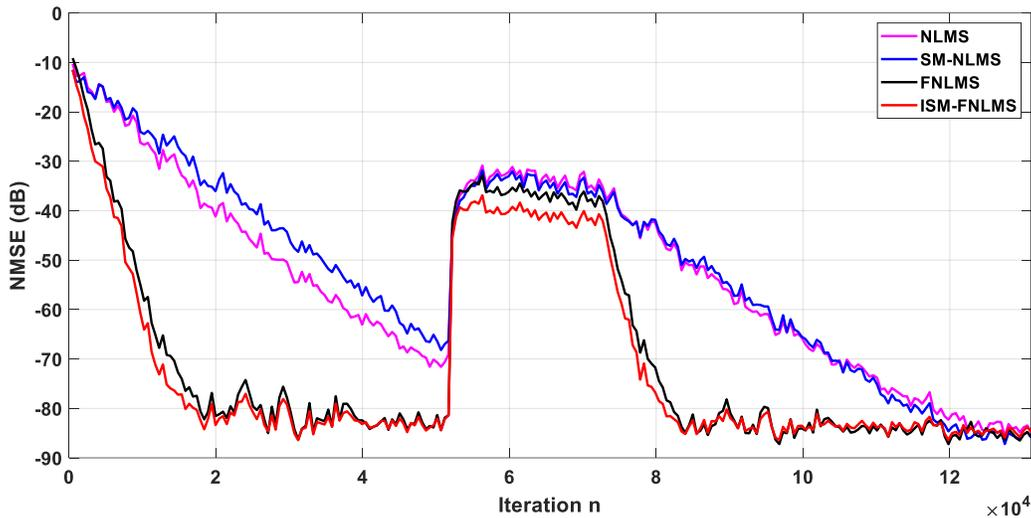
**Figure.2.19.** Comparison of tracking time-varying system of length  $L = 1024$ . Input: USASI noise. No output noise.
