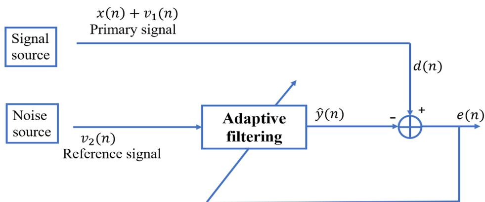
Figure 1. 7: The bloc diagram of noise cancellation.
