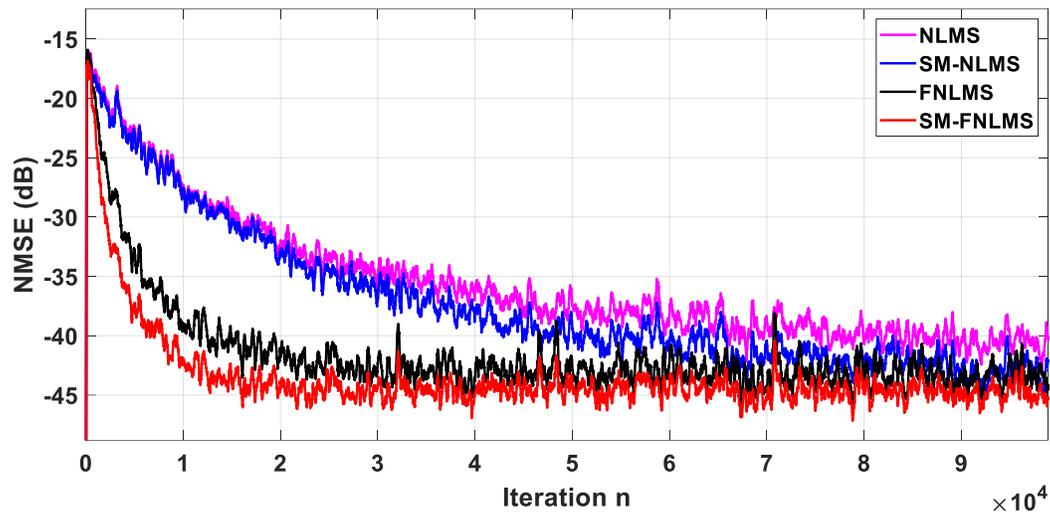
**Figure.2.4.** The Comparison of the initial convergence and the steady-state NMSE. Input: WGN-AR(20) signal with Car system of length  $L = 1024$ . SNR=50 dB.
