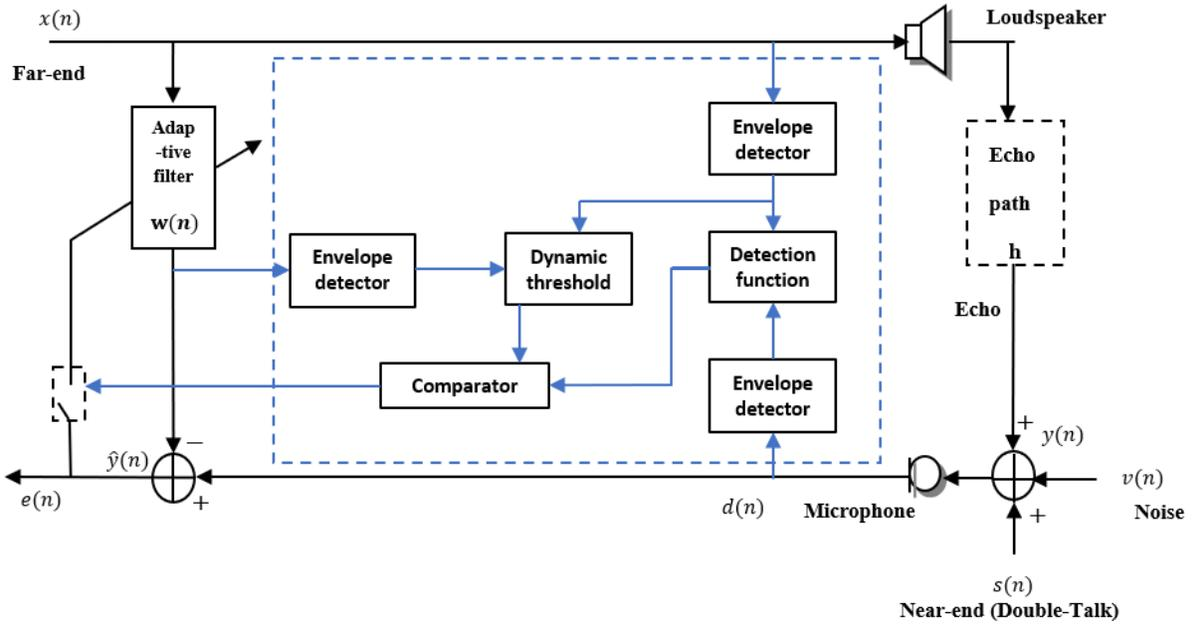
**Figure.3.3.** Bloc diagram of the AEC with DTD based on the signal envelope [46].
