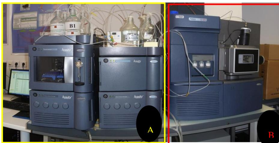
**Figure 20 :** (A) Chromatographe liquide ultra haute performance, ACQUITYTM.
