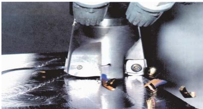
Figure 18: Broutement a cause de vibration
