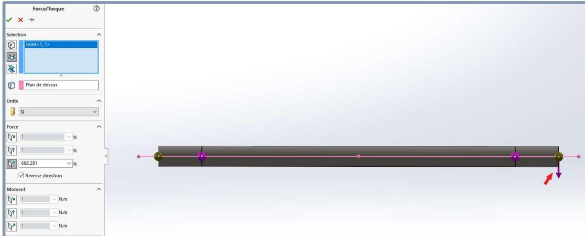
*Figure 4.6: The applied force on the shaft*
