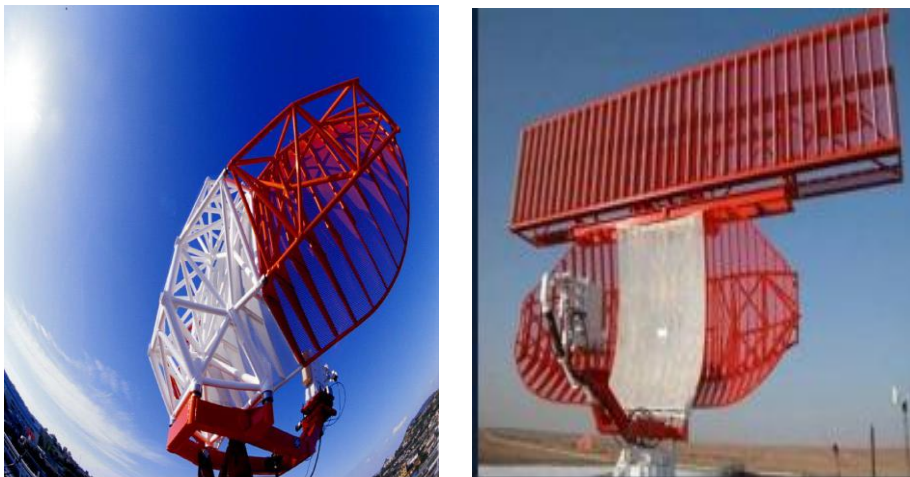
Figure II.4 : Antenne radar ATCR 33S.
