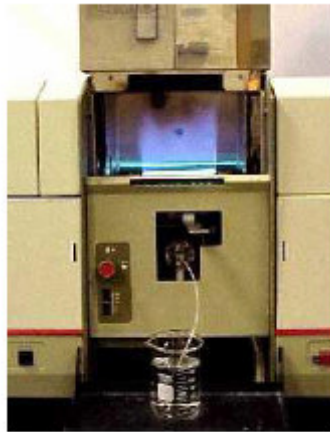
Figure II.7 : La flamme – atomisation.
