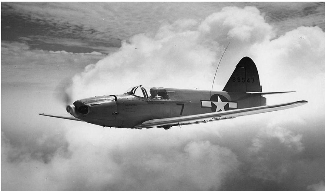
**Figure I-6:** US Navy Culver TD2C-1 target drone © US Navy National Museum of Naval
