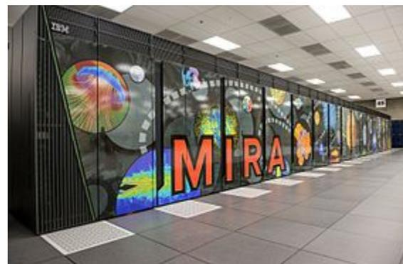
Figure 1.2: Blue Gene/Q supercomputer ("Mira")
