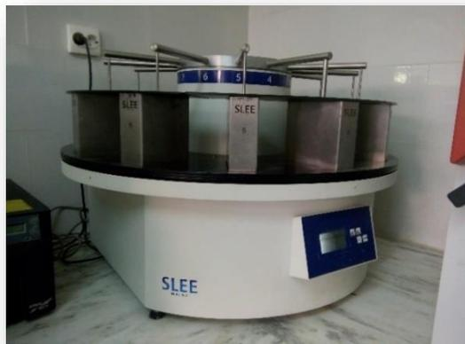
**Figure 16 :** Automate de coloration (photo original).
