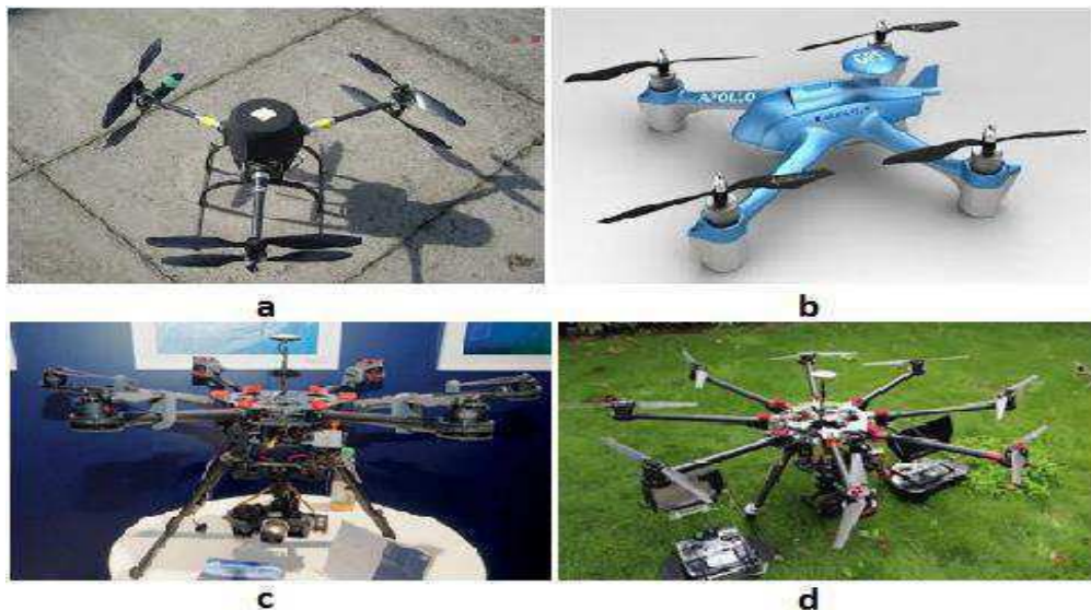
Figure. 1.9: a- Drone tri-rotor. b- Drone QUADRIROTOR. C- Drone HEXACOPTERE. d- Drone OCTOCOPTERE.
