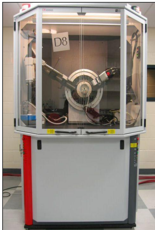
Figure : Diffractomètre de type Bruker ADVANCE 8
