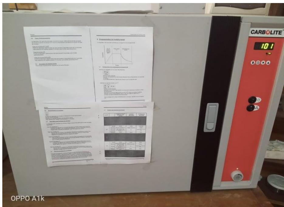
Figure II. 5: Etuve de type CARBOLITE PF 60.
