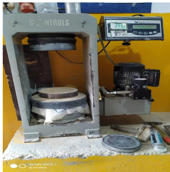
Fig. 3.11: Presse hydraulique (2000 kN).
