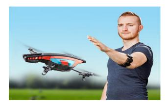
**Figure (I-7):** *Controlling the UAV using gestures.*
