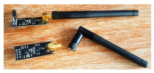
**Figure (IV-7):** *NRF24L01+ module*
