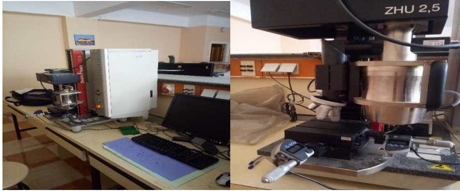
Figure II.9. Instrument de micro-indentation Vickers.
